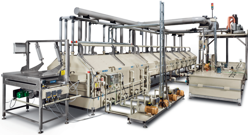
Backside of ultrasonic cleaning plant.
