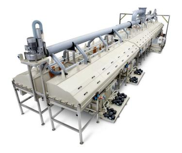
View of plating plant for 8 individual wires
